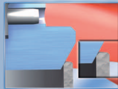
1. "Cut off effect" – the conical shape of the marginal seat causes surface deposits to be removed during sealing
