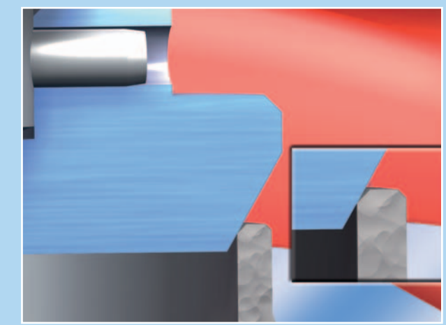
1. "Cut off effect" – surface deposits are removed from the seat when the valve closes
